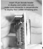
Mount the 14 pin female header on the display module soldering only one pin. Then verify the connector is at a right angle to the module, remelting the soldered pin and adjusting the connector if necessary.
