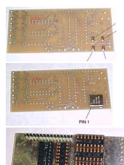
Begin by placing solder globs on the four rectangular pads for the surface mount TCXO. If I pre-installed the TCXO, I could not test it. If unit displays only 8 black squares then check and reflow the solder on its four corners.
