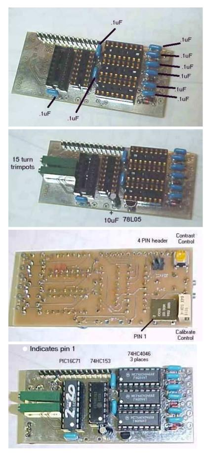
Then install and solder 9 each .1 uF capacitors **Caps can be blue or brown**.
