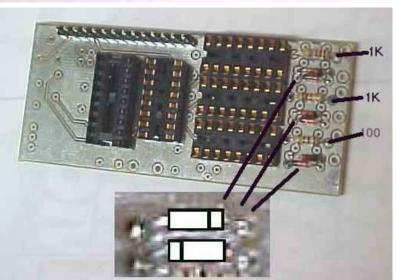
Next install and solder the two 1K and the 100 ohm resistors and the six back to back diodes.
