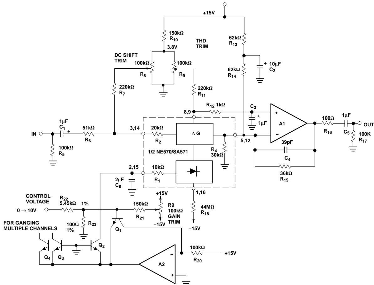
Figure 16. Voltage-Controlled Attenuator
