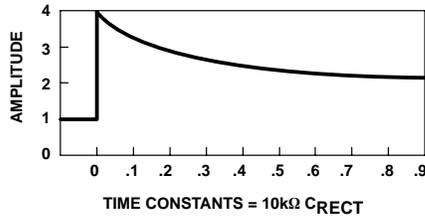
**Figure 10. Compressor Attack Envelope +12 dB Step**
