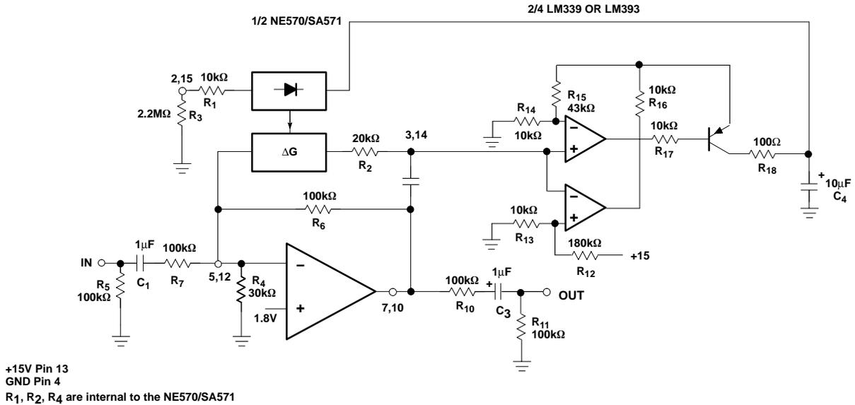
Figure 12. Fast Attack, Slow Release Hard Limiter
