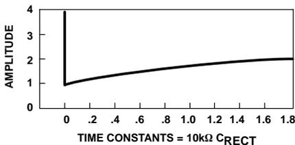
**Figure 11. Compressor Release Envelope -12 dB Step**
