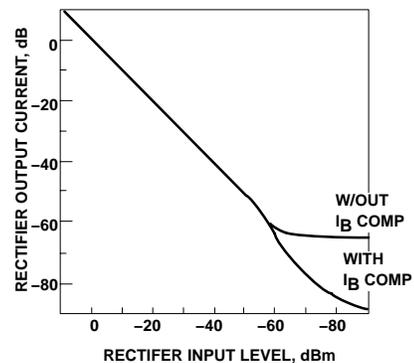
Figure 8. Rectifier Performance with Bias Current Compensation
