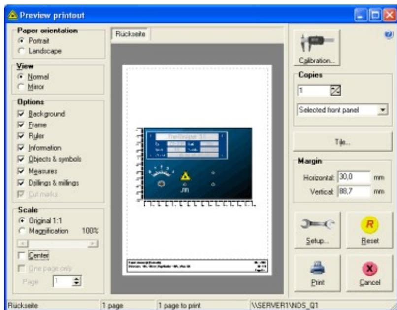
The preview depends on the selected paper format of your printer. As long as the option CENTER is checked, the printout is adjusted to the centre of the paper automatically, otherwise you can drag and drop the printout in the preview to the desired position. The MARGIN values measure the distances between the left/top corner of the front panel (frame) and the physical paper edges. You can enter exact margin values to the edit fields as well, to determine the print position.
