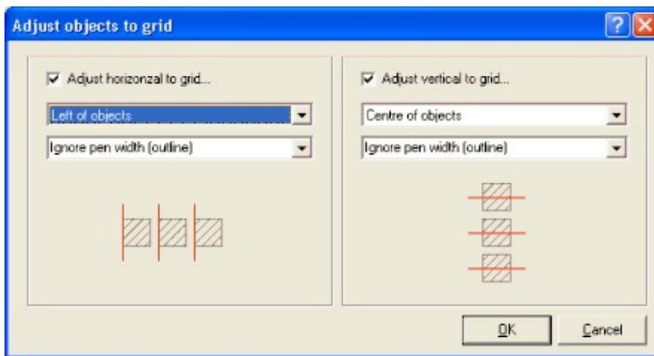
Adjustment can be made in horizontal or vertical direction. You need to specify which point of the object is forced on the grid: Left (top), right (bottom) or centre. The objects pen with can be considered or ignored for calculations. A schematic diagram in the dialog explains the selected options.
