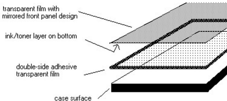
You may also find single-side adhesive films, sold by some electronic suppliers, that can be used with printers. These films are applied directly on the front panel and finally protected with a second transparent, self-adhesive film.
