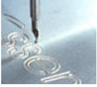
Font panels often have cuttings for switches, instruments, etc.. You can assign a milling tool or an engraving tool – instead of a pen - to any contours that have been drawn with the functions line, circle, rectangle, polygon, text etc. This is done in the PEN administration with the three corresponding buttons.
