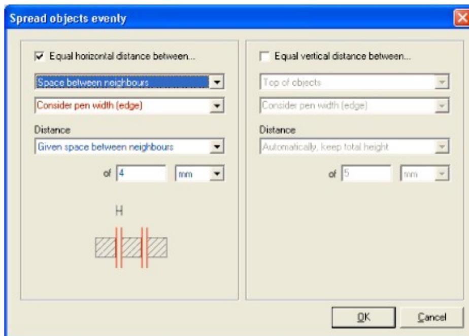
Some setting must be made for this function. Objects can be spread in horizontal and vertical direction. First of all you need to specify which distances shall be made equal:
