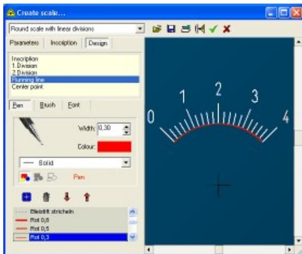
You can click on DESIGN to change pen, brush and font of the scale individually. A list shows the components of the current scale (1. Division, 2. Division, Centre point, etc.). This list is used to select the components that you want to modify. You can select one or more entries of the list. (To select more than one object, hold down SHIFT during selection.)
