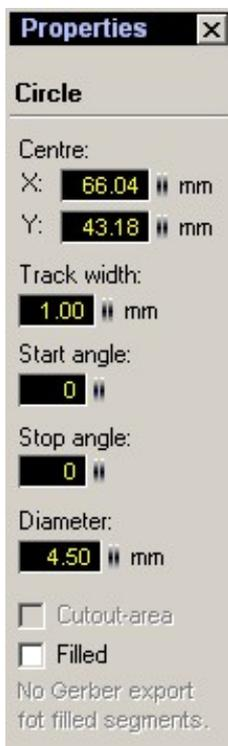
During the input of the diameter note that you must include the width of the drill. Since the tool will mill concentrically around the radius, the milled hole width will be wider. You must take the milling tool width off from the diameter of the hole, in order to obtain the correct hole width result. In our case we want a hole of 5,5mm and our milling tool has a width of 1mm. The input in the circular
