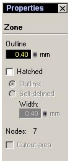
A zone must not have a solid filling. You can select Hatched to create a hatched filling.
