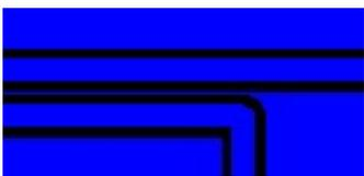
Figure: Narrow copper area between tracks.
