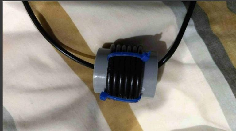
***Recommendation: For homebrew antennas, use coil if you’re primarily a CW operator, don’t use coil if you’re primarily a SSB operator. Or leave it out and use “touch-up” antenna tuner.***
