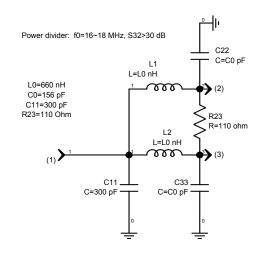
Figure 4 shows the schematic of the combiner
