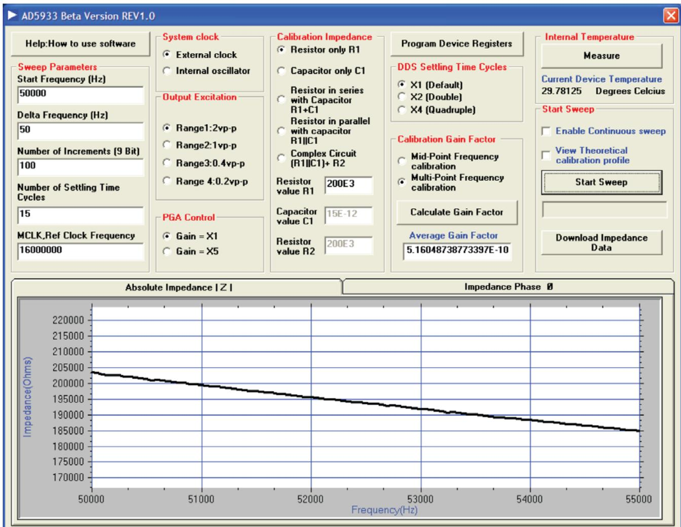
Figure 3. Measuring the Impedance of Capacitor
