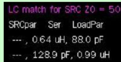
For example, to calculate the corresponding LC 50 Ohms at 17.5 MHz is 0,64uH, 88pF or 128,9pF, 0,99uH. In AA, it shows the following diagram on the right side of the screen.
