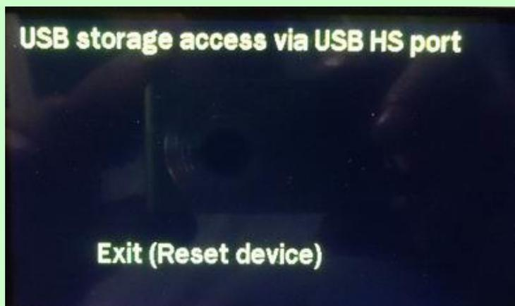
**Working with «AntScope» program** - only in the main menu mode. The device connects to the PC through the left USB-connector (mini-USB). Driver installation is required for the board STM32-Disco. After starting the program in its settings, you must select the COM port.
