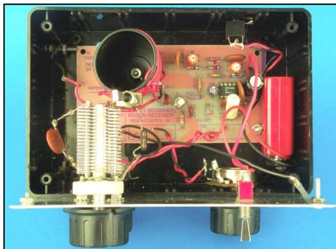
In this version of the receiver, a prototype PC board is used; it is not directly representative of the currently produced board, although they are similar. In this view of the receiver, the antenna has been removed. The TUNING capacitor is at the left. Immediately behind the capacitor is the coil, L1. Attached between the TUNING capacitor and the VOLUME control pot immediately beneath you can see D1, C4 and R4 as discussed in the text.
