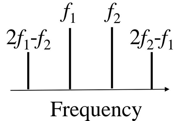
**Jammer Signal Emission to Adjacent Channels**
