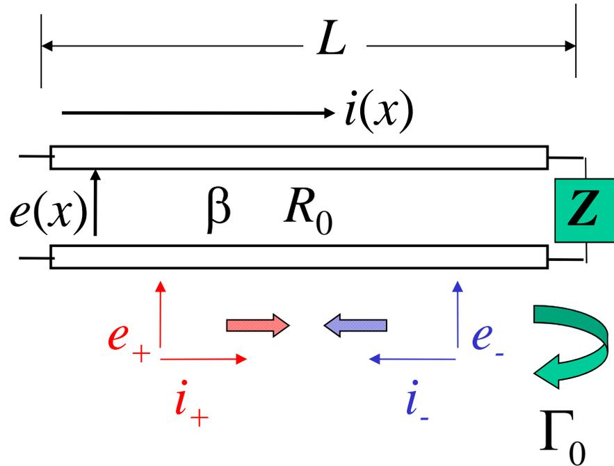
$$\Gamma_0 = \frac{e_-}{e_+} = \frac{Z - R_0}{Z + R_0} = \frac{G_0 - Y}{G_0 + Y}$$
