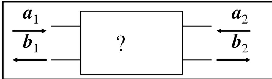
$$\begin{pmatrix} b_1 \\ b_2 \end{pmatrix} = \begin{pmatrix} S_{11} & S_{12} \\ S_{21} & S_{22} \end{pmatrix} \begin{pmatrix} a_1 \\ a_2 \end{pmatrix}$$
