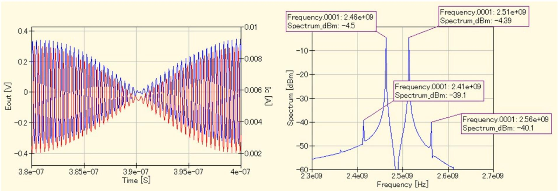
$$P_{2a \pm b} [\text{dBm}] = 2 \times P_a [\text{dBm}] + P_b [\text{dBm}] - 2 \times \text{OIP3} [\text{dBm}]$$
