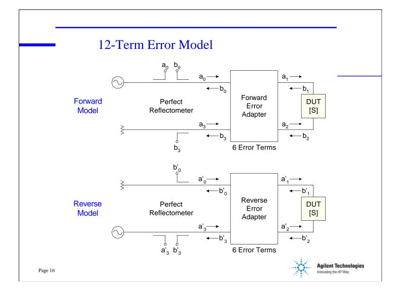
The two-port case can be modeled in the same manner as the oneport. A fictitious error adapter is placed between the two-port DUT and the 'perfect reflectometer' measurement ports. This error adapter contains the 6 error terms for the forward direction. A similar 6 term model is used in the reverse direction.
