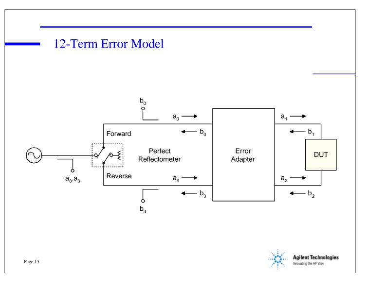
Many of the older and lower cost network analyzers use three couplers instead of four. This puts the switch between the couplers and if the switch characteristics change as the switch is changed the error adapter's error terms will change. Even some four coupler network analyzers use this method as well, choosing not to use the fourth coupler.
