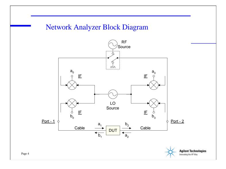
This is a generic block diagram of a 4 channel network analyzer. The source can be switched to excite port-1 or port-2 of the device under test (DUT). The switch also provides a  $Z_0$  termination for the output port in each direction. Directional couplers are used to separate the incident, reflected and transmitted waves in both the forward and reverse direction. Mixers are used to down convert the RF signals to a fixed low frequency IF. The LO source is tuned to the frequency of the RF + IF.
