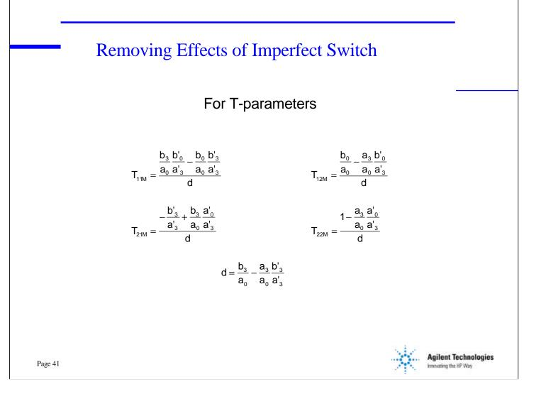
The same approach can be used for measuring the t-parameters. This will also remove the effects of the switch and requires 6 ratio measurements.
