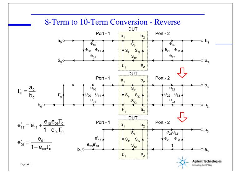
The same procedure can be used for the reverse model. There is a constraining relationship for the 8-term and 10-term models. This is the same as saying that the 8-term model can reduce to 7 terms when making ratio measurements. And the 10-term model can reduce to 9 terms.
