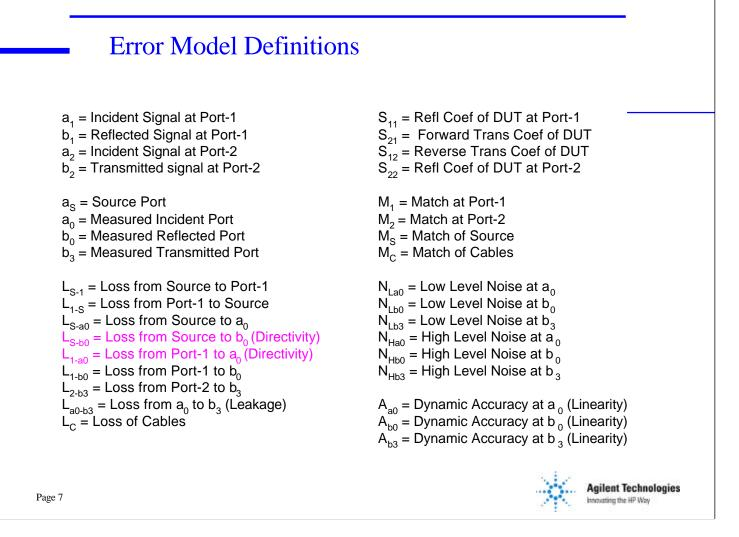
The above table gives the description of each of the branches and the key nodes for the flow graph. This provides a very complete model for the network analyzer. However it is possible to reduce the flow graph without any loss in accuracy. This reduced flow graph is much easier to analyze and will be discussed next.
