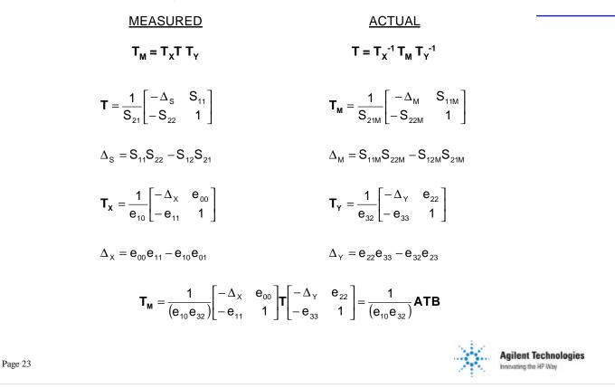
Note that the flow graph is a cascade of the input error box (X), the DUT, and the output error box (Y). The measured result of this cascade is most easily calculated by using the cascade matrix definition (t-parameters).
