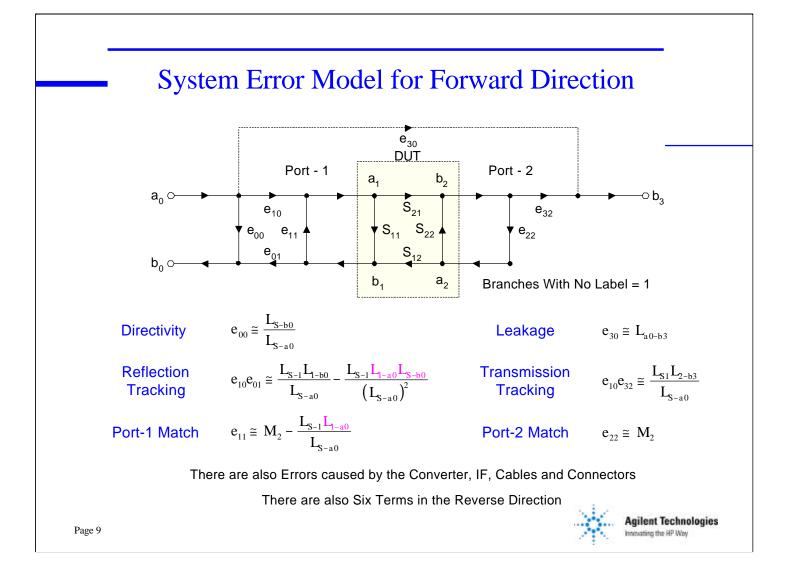
The resultant system error model is the forward portion of the well known 12-term error mode. Each of the branches have an accurate relationship to the original hardware oriented flow graph presented earlier. The 6 forward terms described above show a simplified set of equations relating the two flow graphs.
