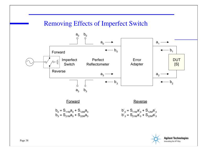
As stated earlier there is a technique to ratio out or remove the effects of an imperfect switch. Note that the measurement channels are all on the DUT side of the switch. This allows the measurements of incident and reflected signals from the switch. Then we can use the reflectometers to measure the reflection and transmission of the switch and effectively 'remove' the switch from the system.
