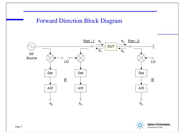
This block diagram shows the measurement system switched to the forward direction. Each of the IF signals are detected and digitized and the real and imaginary terms are measured. From this data the magnitude and phase can be calculated.
