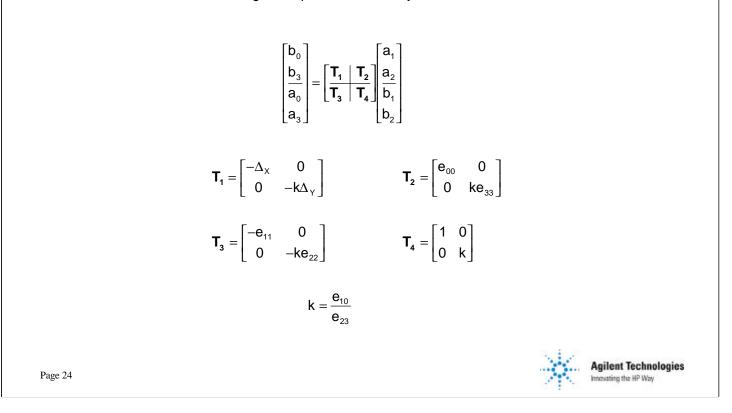
There is another mathematical formulation for the 8 term error model. Consider the error adapter as just one adapter between the perfect measurement system and the DUT. Then model this error adapter using the cascade t-parameters. This t-parameter matrix (T) can be partitioned into the four sub matrixes  $T_1$ ,  $T_2$ ,  $T_3$ , and  $T_4$ . The 7 error terms are now defined as  $\Delta_X$ ,  $k\Delta_Y$ ,  $e_{00}$ ,  $ke_{33}$ ,  $e_{11}$ ,  $ke_{22}$ , and k.
