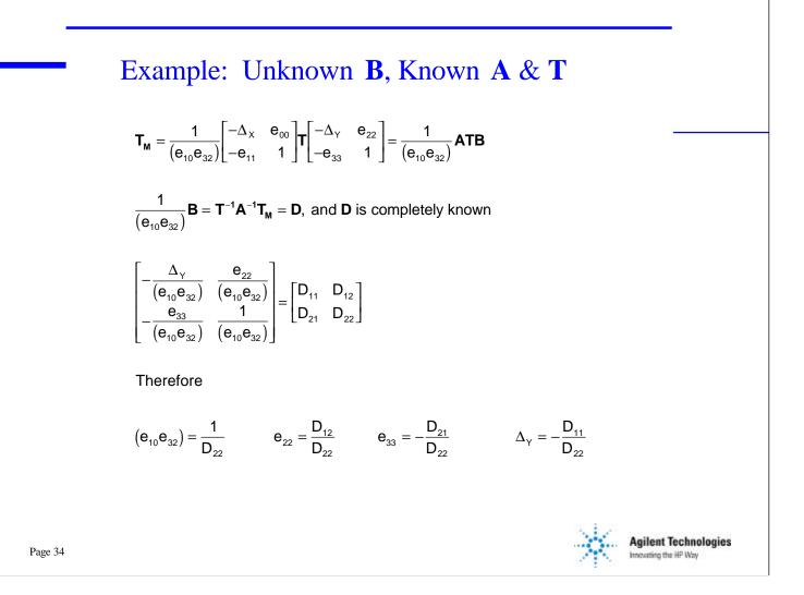
This example calibration approach (TXYZ) requires 3 known standards on port-1 but none on port-2 as long as the thru connection is known. The known thru connection provides 4 observations. The 3 known reflection standards connected to port-1 complete the required 7 known conditions.
