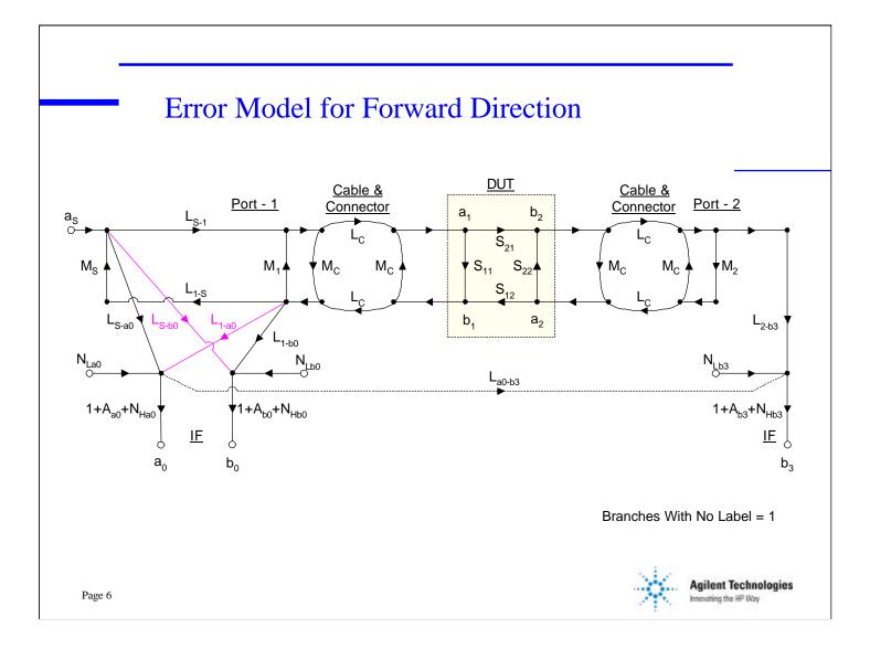
From the block diagram a flowgraph can be developed showing all the possible signal paths. These paths not only include the main desired signals but the loss, match errors, and leakage errors, of the network analyzer along with the cables, connectors, or probes that connect to to DUT.
