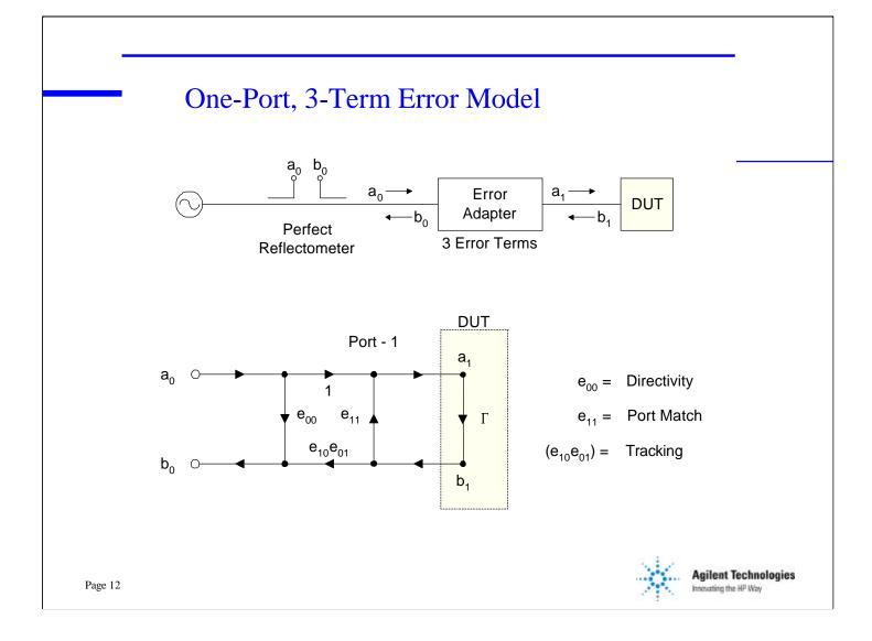
The one-port calibration procedure will now be described. The 12term model described earlier simplifies considerably when a oneport device is being measured. The model simplifies to just the terms describing the directivity, port match , and tracking errors at each port.
