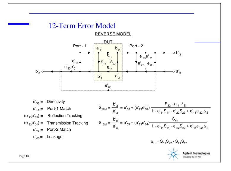
Solving the reverse flow graph yields measurements  $S_{22M}$  and  $S_{12M}$ . These two equations contain all four actual s-parameters of the DUT and the six reverse error terms.
