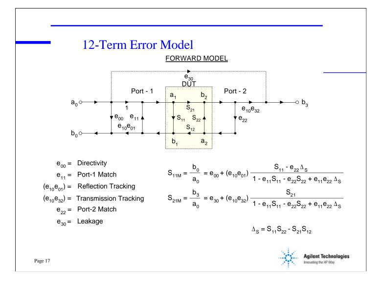
Solving the forward flow graph yields measurements  $S_{11M}$  and  $S_{21M}$ . These two equations contain all four actual s-parameters of the DUT and the six forward error terms.
