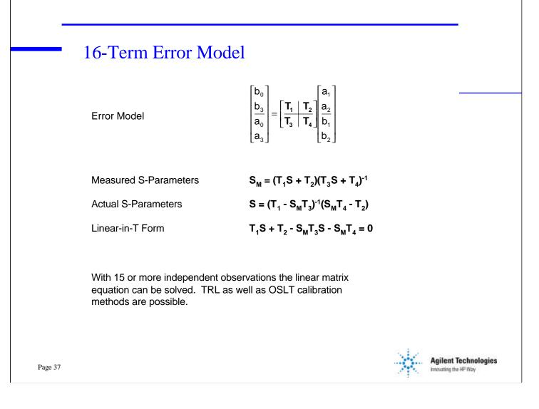
Solving the 16-term model can be done the same way that the 8term model was solved. In the 8-term model there were 8 zero terms in the T matrix with the assumption of no leakage. For the 16-term model all terms are present. Of course the set of resultant linear equations contain more error terms, but the approach is the same.
