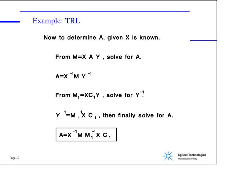
The unknown device characteristics can be easily calculated by knowing the parameters of the X error adapter, the known standard  $C_1$ , and the measured data of the test device and measured data for  $C_1$ .
