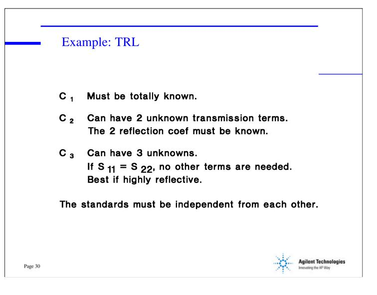
All 4 parameters of  $C_1$  must be known but only 2 parameters for  $C_2$ and none for  $C_3$  if  $S_{11} = S_{22}$ . The simplest of all standards is a through line, so let  $C_1$  be a thru and  $C_2$  a  $Z_0$  matched device. If needed, impedance renormalization can be used to shift to a different impedance base. The other parameters of  $C_2$  and  $C_3$  can be solved from the data.
