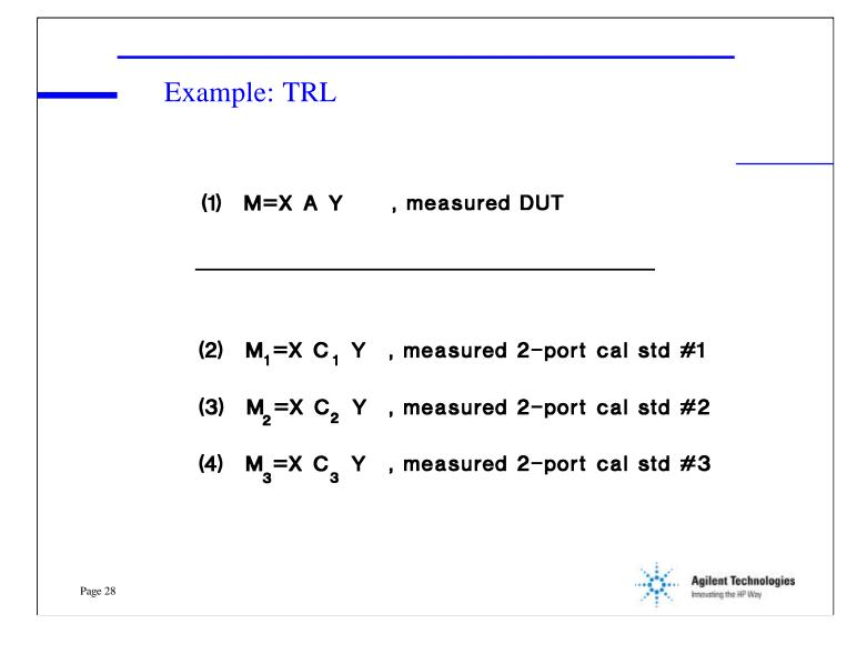
It is convenient to use t-parameters because it allows one to represent the overall measurement, M, of the DUT, A, as corrupted by the error adapters as a simple product of the matrixes,
