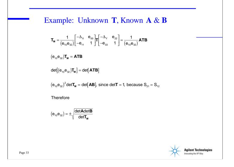
This example is for the unknown thru calibration method (UXYZ). This is most easily developed using the cascaded t-parameter formulation. With 3 known standards at port-1 and port-2, 6 conditions are provided. The thru standard with  $S_{21} = S_{12}$  provides the 7th required condition. The key to solving this approach is that the determinant of T is unity for the passive thru calibration connection ( $S_{21} = S_{12}$ ).
