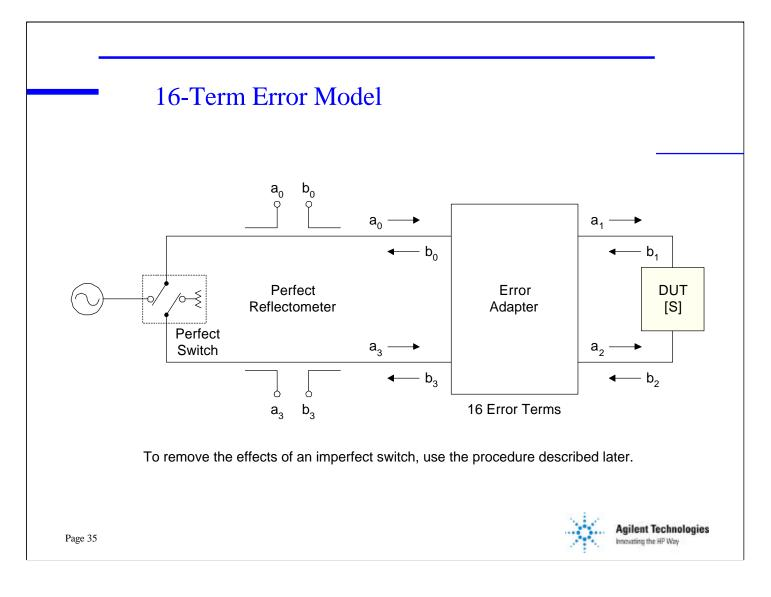
With the 8-term model we assumed that there was no leakage between the various measurement ports. The 16-term model makes no assumptions about leakage.
