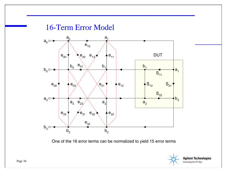
These leakage terms add 8 additional error terms to the model. Not only is the traditional crosstalk term included, but switch leakage, signals reflecting from the DUT and leaking to the transmission port, common mode inductance, and other leakage paths are included. In a coaxial or waveguide system, assuming the switch has high isolation, these errors are small. But in a fixtured or wafer probe environment these errors can be much larger.
