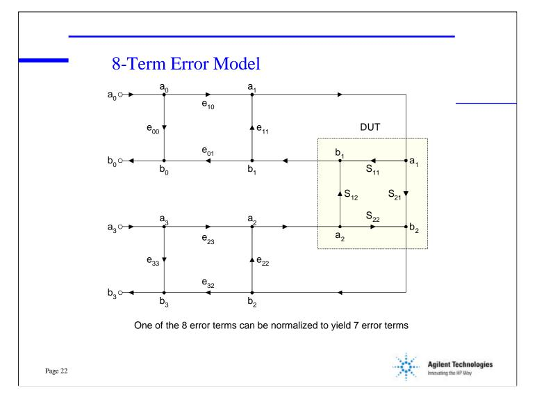
The flow graph consists of an error adapter at the input and output of the DUT. For ratio measurements of s-parameters, the number of error terms is reduced to 7 since the error terms can be normalized.
