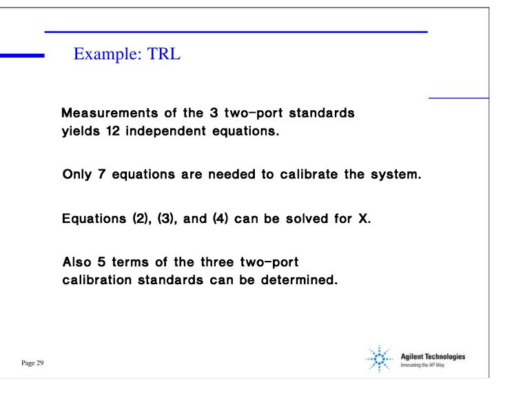
While there are 7 unknowns, measuring three 2-port standards yields a set of 12 equations. Due to this redundancy, it is not necessary to know all the parameters of all the standards. X and Y can be solved for directly plus 5 characteristics of the calibration standards.
