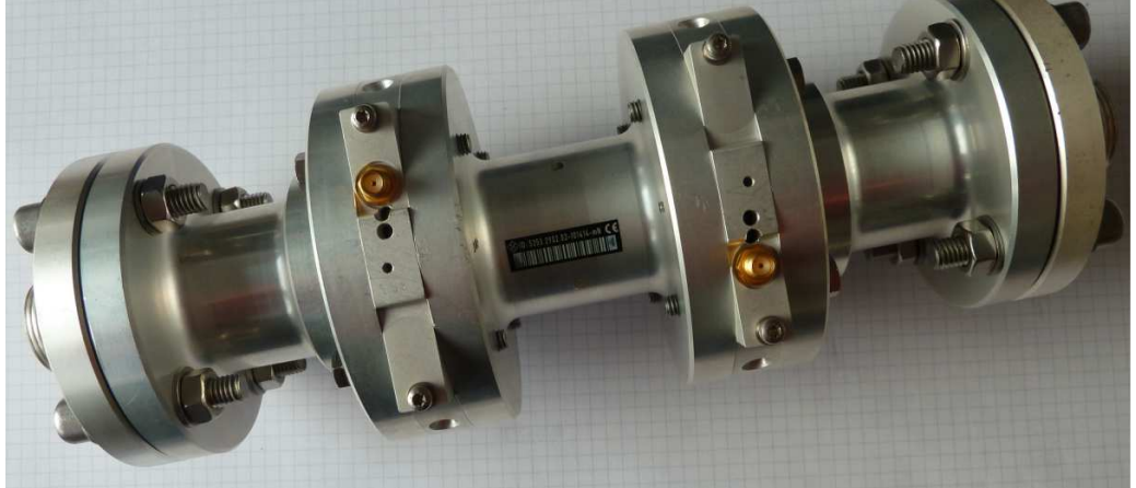
Fig. 13: Broadband directional coupler, 9 kHz to 250 MHz.
