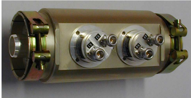
Fig. 10: Directional coupler with two measuring systems and air line connection.
